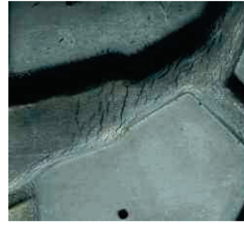
Cracking Between Tread
