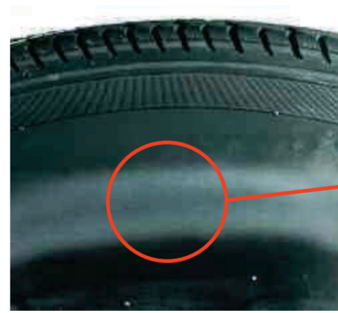
Under-Inflated tyre - An abrasion may run around the circumference of the tyre and wrinkles may be observed in the inner liner.
