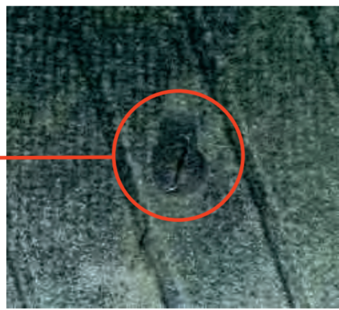
Puncture - Normally, the only evidence of a puncture will be a cut that extends from the tread of the tyre through the inner liner.
