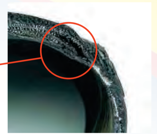
Shoulder Separation - A groove worn in the shoulder of the tyre is usually evidence of separation.
