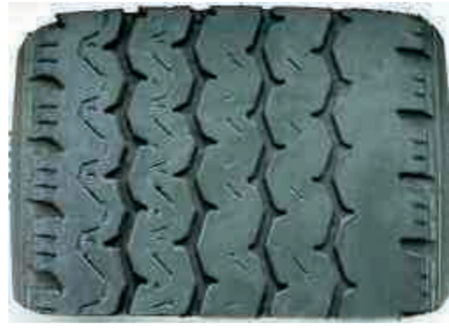
Rapid Shoulder Wear
