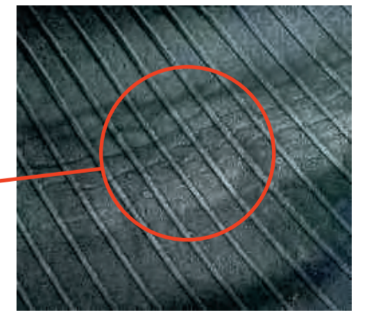
Under-Inflated tyre - An abrasion may run around the circumference of the tyre and wrinkles may be observed in the inner liner.
