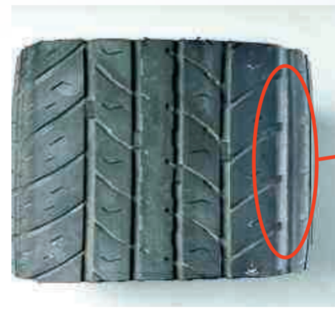
Shoulder Separation - A groove worn in the shoulder of the tyre is usually evidence of separation.
